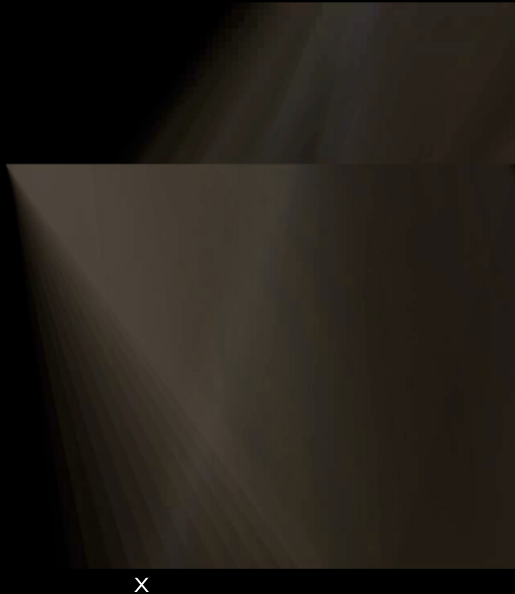
one scanline with different focal distances, i.e. one slice from a focal stack
