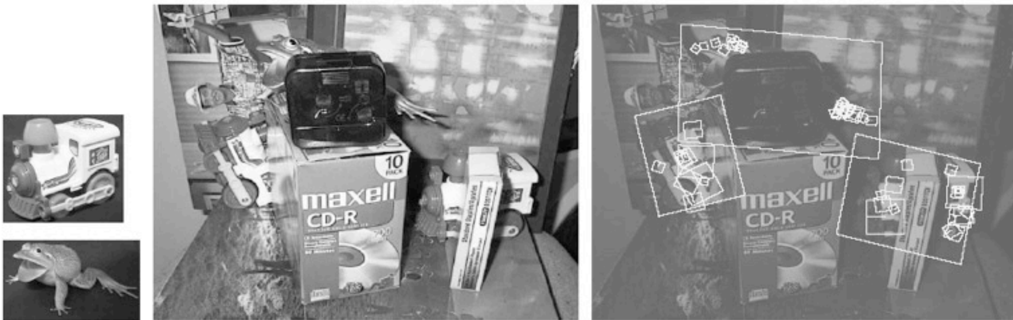
Figure 12: The training images for two objects are shown on the left. These can be recognized in a cluttered image with extensive occlusion, shown in the middle. The results of recognition are shown on the right. A parallelogram is drawn around each recognized object showing the boundaries of the original training image under the affine transformation solved for during recognition. Smaller squares indicate the keypoints that were used for recognition.
