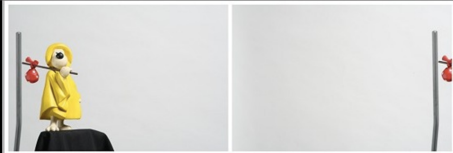
Figure 3. Configuration to reveal the presence or absence of parallax. The subject is first placed at the left side of the frame, and subsequently at the right side after rotation of the camera about a vertical axis with the help of a panoramic tripod head.
