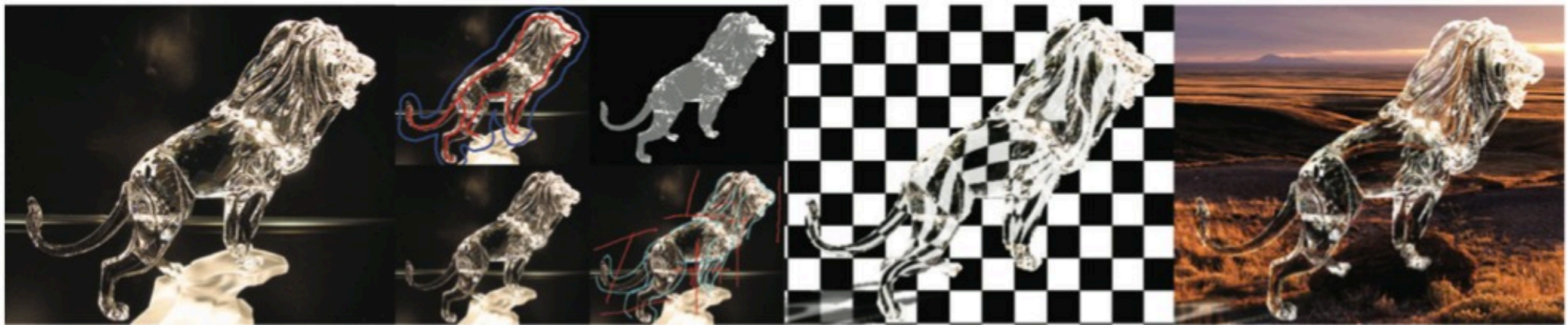
Fig. 1. Attenuation-Refractive Matte (ARM). From left to right: input image (courtesy of Francesco Dazzi), casual markup, ARM, and the composite completed with simulated Fresnel effect and caustic shadow.
