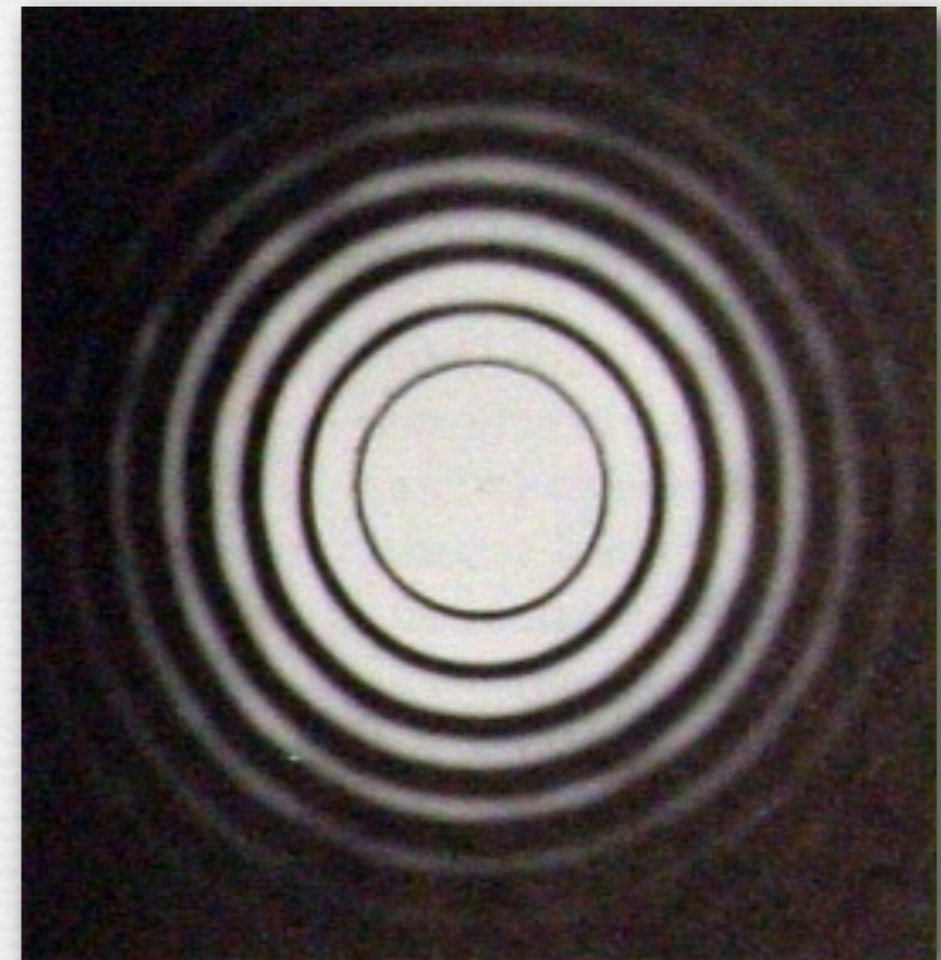
diffraction from a circular aperture: Airy rings
